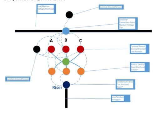
The simple point feature in ArcGIS is expanded to a highfidelity device in the Utility Network model. The composition, location and associations of the individual assets within an assembly are controlled by an XML file that is used by the ElectricDistributionAssemblyBuilder custom transformer in the electric migration workspace.
